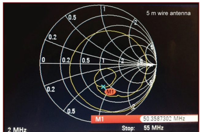
▲ Fig. 13 Measured S_{11} of a 5 m wire antenna with 8 m ground wire, 2 to 55 MHz.
