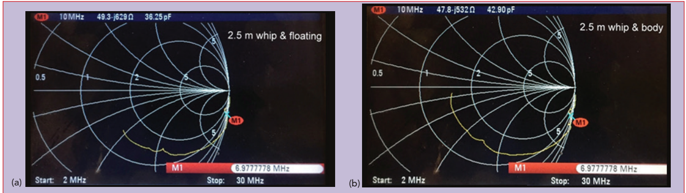
▲ Fig. 18 Measured S_{11} of a 2.5 m whip antenna with floating ground (a) and ground next to the body (b).
