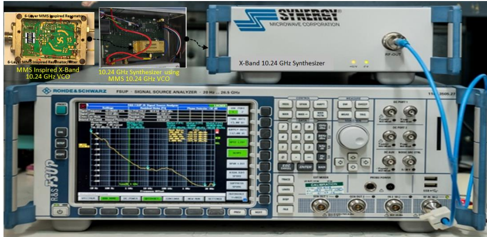
Fig. 2: Phase noise measurement setup: X-Band 10.24 GHz synthesizers using MMS inspired Oscillator
