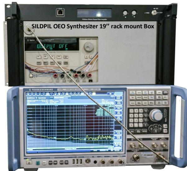
Fig. 8: shows the Rohde & Schwarz FSWP phase noise measurement setup, SILDPIL OEO synthesizer in 19-in. rack-mount enclosure for portability, the size can be reduced based on applications
