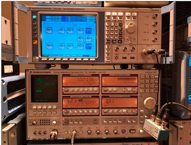
Figure 7: Test setup for receiver intermodulation measurements
