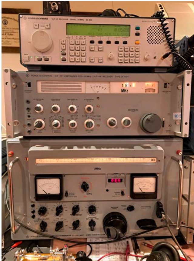
Figure 1: Three generations of shortwave receivers. EK07/D2 HF receiver (bottom) and EK056/4 and EK896 (above), connected to the same antenna for comparison
